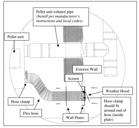
hose clamp around this end of the hose. Once the clamp and screen are installed, the hose should fit snugly in the hole of the outside wall plate, with the hose clamp on the inside of the wall plate and the screen on the outside of the wall plate.
