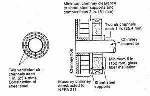
C Sheet steel chimney connector, minimum 24 gauge in thickness, with a ventilated thimble, minimum 24 gauge in thickness, having two 1-in. air channels, separated from combustibles by a minimum of 6-in. of glass fiber insulation. Opening shall be covered, and thimble supported with a sheet steel support, minimum 24 gauge in thickness.
