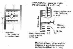
A Minimum 3.5-in thick brick masonry all framed into combustible wall with a minimum of 12-in brick separation from clay liner to combustibles. The fireclay liner shall run from outer surface of brick wall to, but not beyond, the inner surface of chimney flue liner and shall be firmly cemented in place.
