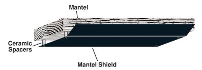
3. Then use another hole in the Mantel Shield as a pilot to drill a
